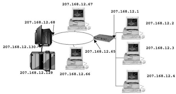
Figure 5-25. Installing TCP/IP Direct Connect into Network
